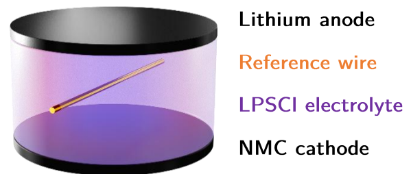
Figure 1. Sketch of the components comprising the three-electrode cell stack.
