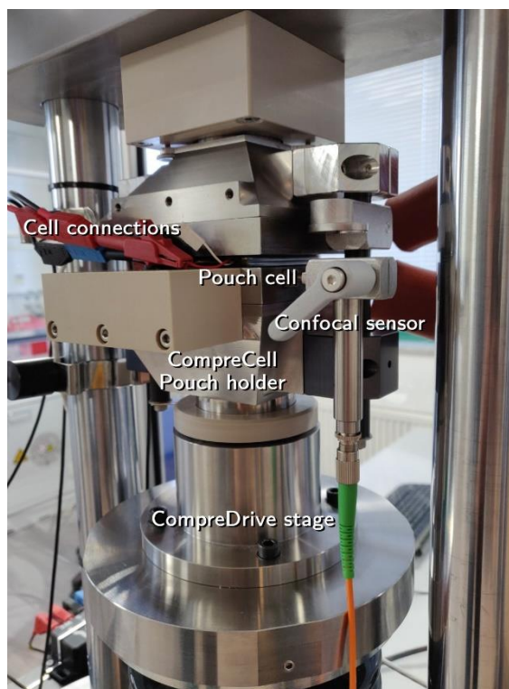
Figure 2. Experimental setup with the pouch cell mounted in the CompreCell Pouch cell holder within the CompreDrive.
